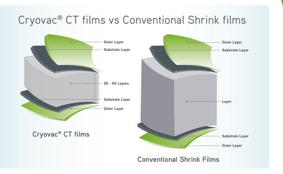
Cryovac® CT series of films provides a radical new technological capability within the packaging industry. This patented innovation incorporates up to 50 discrete microlayers compared to conventional shrink films, which are typically comprised of 1, 3 or 5 layers.
